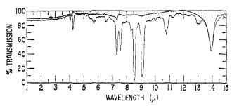
Figure 4. Infrared spectrum of perfluoromethylacetylene.
